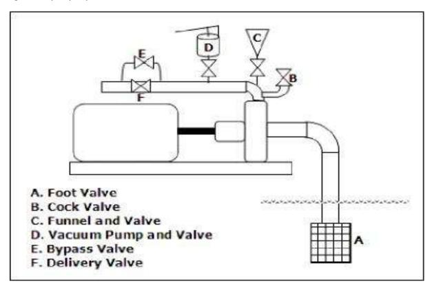
If the pump is above the water level, the pump can be primed using the funnel, the vacuum pump or the line pressure.
