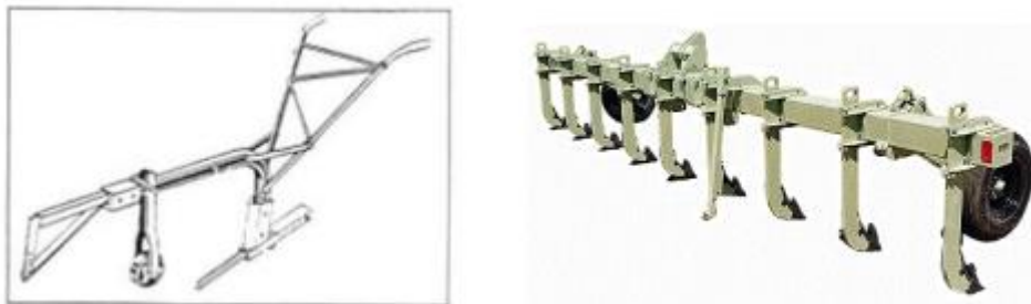
Figure 1.2. A hand-held ripper on the left and a mechanical drawn ripper on the right.
