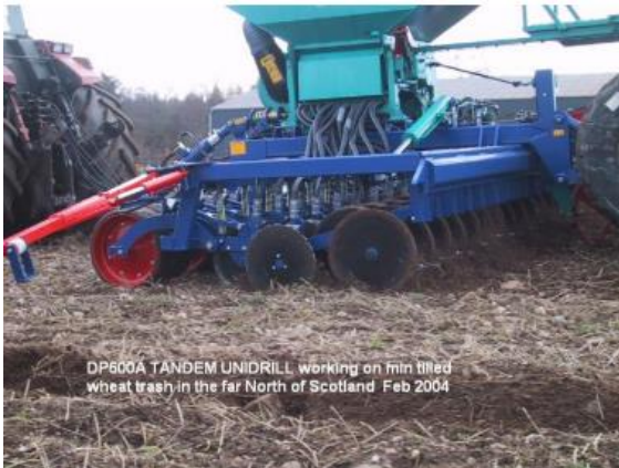
Figure 4.1. Seed drilling (sowing) in minimum tilled soil, covered in wheat mulch.
