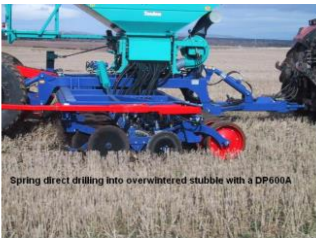
Figure 4.2. Seed drilling (sowing) in a zero tilled soil, covered by the stubble of the previous season's wheat.
