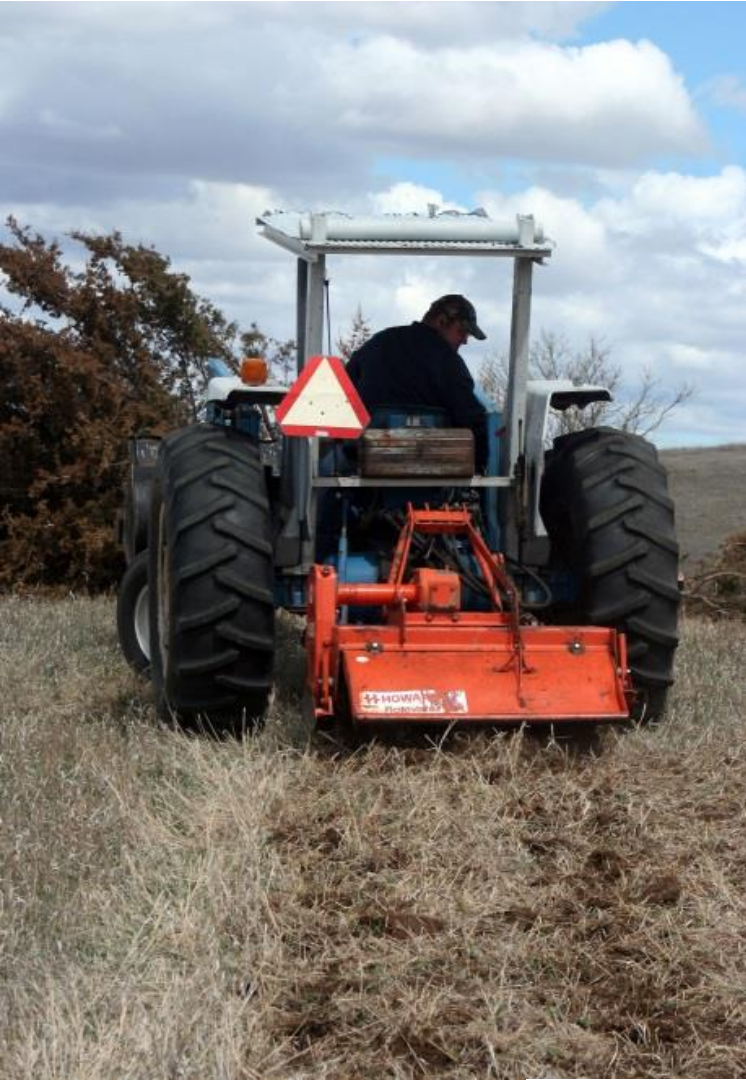
Figure 11. One pass with a tiller might not be enough to expose a solid line of soil through the firebreak.
