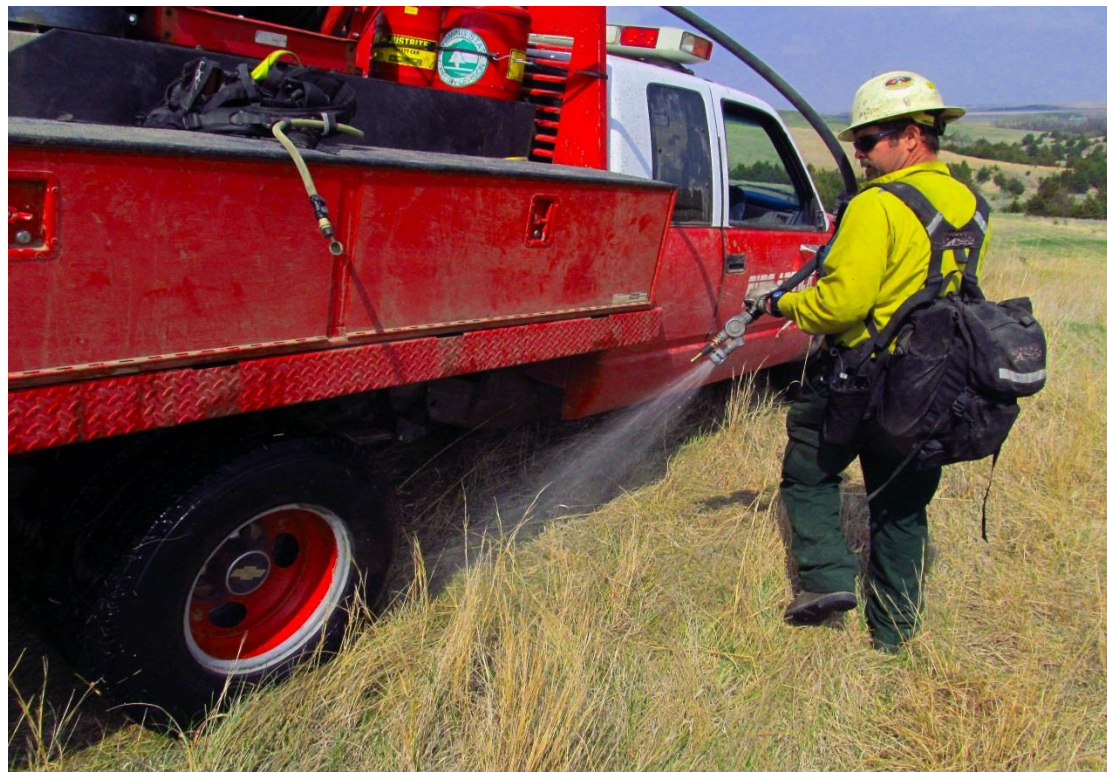
Figure 12. Since they can quickly evaporate, wetlines should only be considered a temporary firebreak. Compacting the vegetation with a tire can increase the performance of a wetline.
