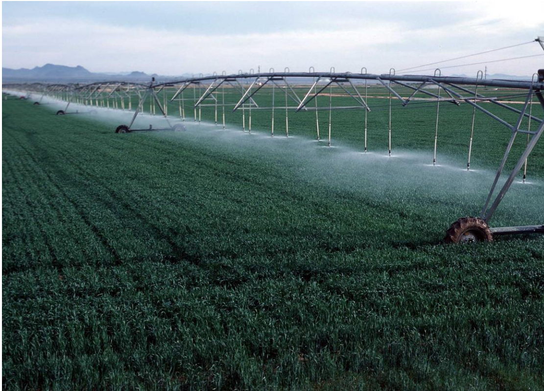
Centre pivot with drop sprinklers.
